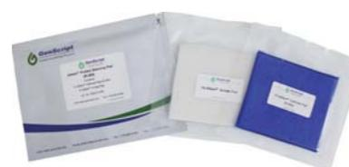
3. Tear the sealing of the 1×eStain® Anode Pad package. Remove the eStain® Anode Pad from the package and place it on the anode plate of the eStain® 2.0 Protein Staining Device.
