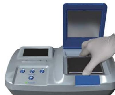
3. Remove the new eStain® 2.0 Graphite Electrode from the packing box.
